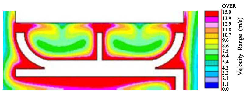
(b) Contour map of peripheral velocity when the ring speed U=37.9\text{m/s} ( R_\omega=7.0\times 10^3 )
