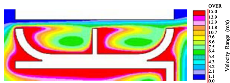
(b) Peripheral velocity when the ring speed U=37.9\text{m/s} ( R_\omega=7.0\times 10^3 )
